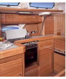
• Easily worked galley with propane stove with oven, front opening refrigerator and storage in enclosed cabinets and lockers
