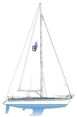
Length overall 46′7″ Length hull 45'11" Length waterline 40' Beam 14'3" Draft standard 6'1" Draft (deep lead option) 6′10″ Displacement 24,250 lbs. **Ballast** 7,275 lbs. Water tank 120 gal. (appx.) Fuel tank 55 gal. (appx.) Main sail & genoa 1,268 sq. ft. (appx.)
